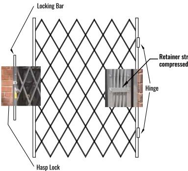
**Retainer strap holds gate** compressed for enhanced access.
